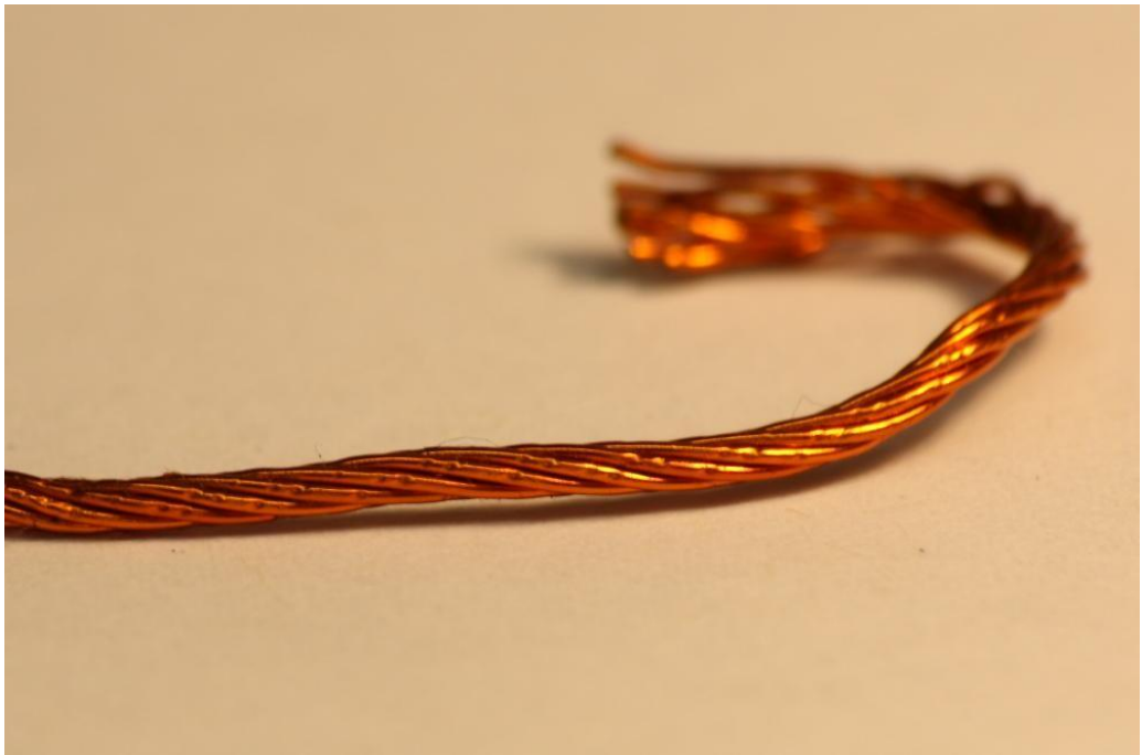
Figure 6-16: Litz Bundle Separated for Submersion in Acetone
