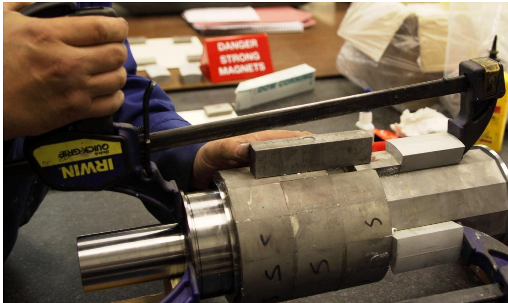
Figure 2-7: Assembly of rotor magnets using a Jig
