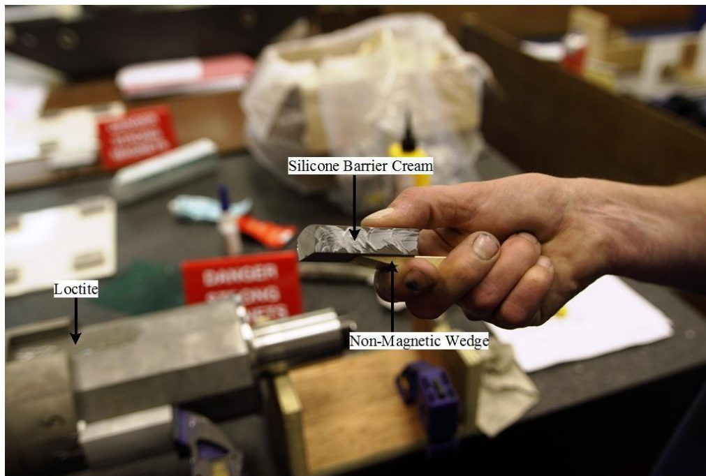
Figure 6-2: Magnetic Assembly Surface Preparation
