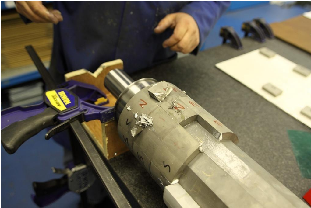
Figure 6-4: Magnet Damage Due to Jumping
