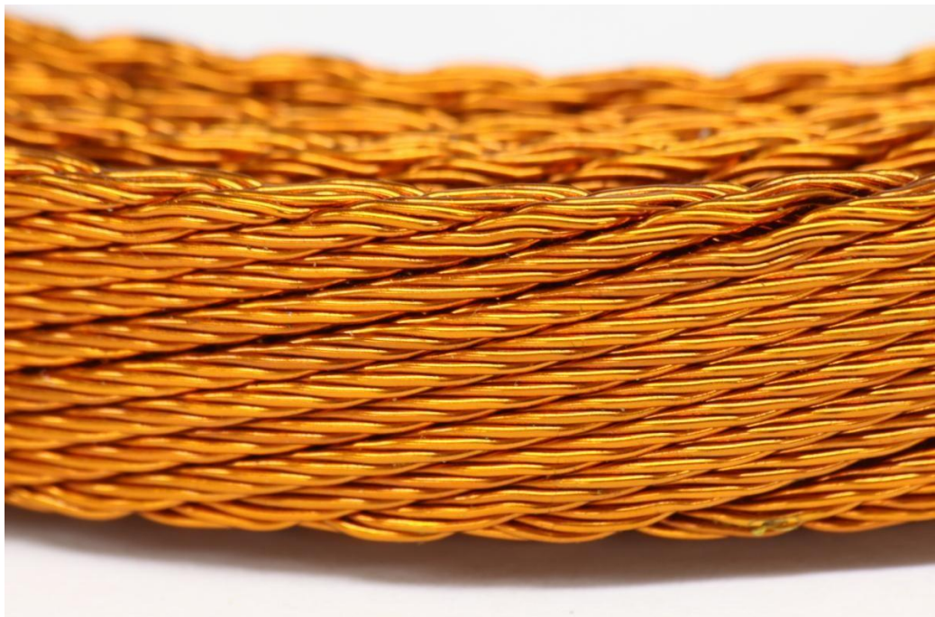
Figure 6-15: Litz Wire used for Solvent Crazing Investigation
